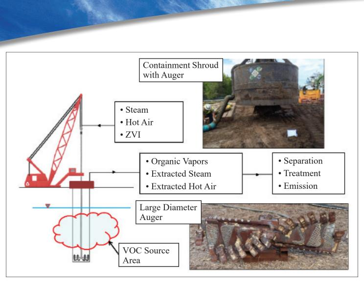
Figure 3. Combined Steam and ZVI Injection (Courtesy of Geosyntec)
